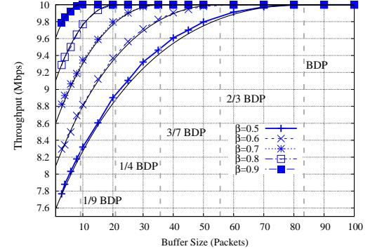
Fig. 1: Throughput of a single NewReno flow, with  $C = 10$  Mbps,  $RTT = 100$  ms (model and simulation).
