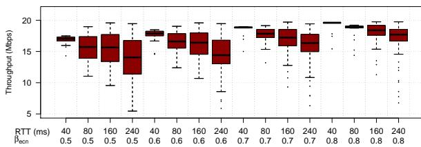
Fig. 8: Throughput improves with higher  $\beta_{\text{ecn}}$ , more so for large  $RTT_{\text{path}}$  (NewReno flow over CoDel,  $C = 20$  Mbps).
